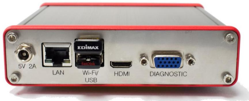
Figure 1. VideoForge HDMI back panel features.
