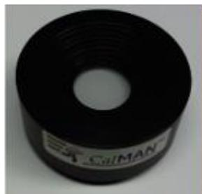
Figure 3. K10-A cosine diffuser.
