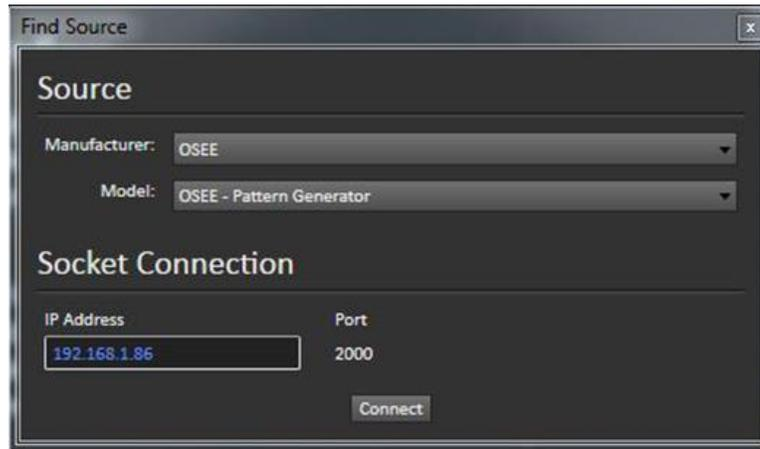
Figure 2. CalMAN Find Source dialog, for connecting to the OSEE monitor internal pattern generator.
