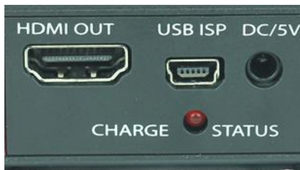
Figure 3. VideoForge PRO top connector panel.
