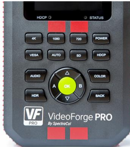
Figure 2. VideoForge PRO buttons & indicators.
