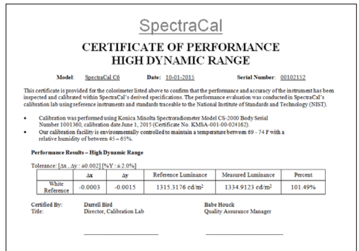
Figure 2: The Certificate of Performance issued with each C6 HDR indicates the meter's luminance and chromaticity accuracy at the tested luminance level.
