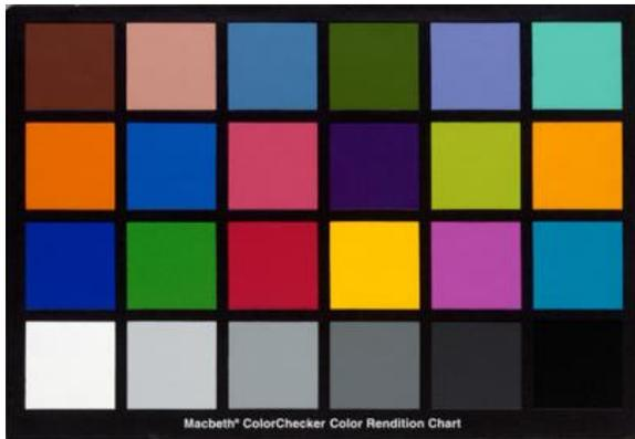
**Figure 8: The ColorChecker chart provides reference colors for visual comparison and for instrument measurements.**
