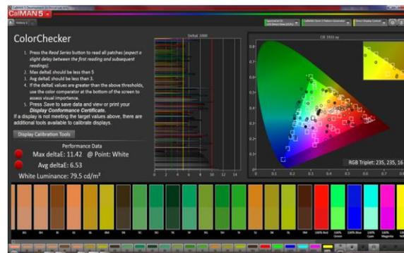
**Fig. 12: CalMAN ColorChecker provides extensive numeric and visual color difference evaluations.**
