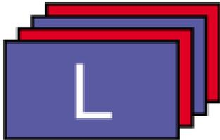
Figure 1: 3D-compatible consumer video displays produce alternating left and right eye image frames for viewing through active shutter glasses.
